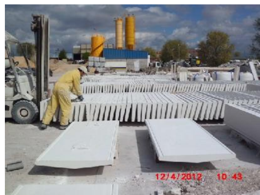
Figure 21. Façade panels containing photocatalytic TiO 2 -sepiolite
