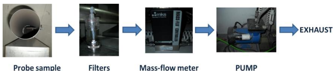
Figure 3. Particle path from the cone calorimeter duct to the exhaust.
