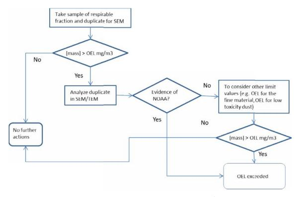
Figure 11. Flowchart describing the procedure to measure mass concentration (mg/m3).
