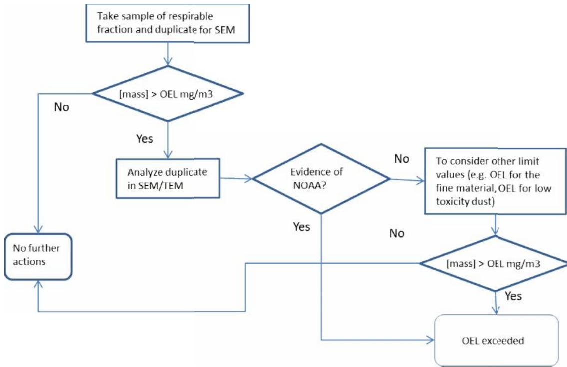
Figure 11. Flowchart describing the procedure to measure mass concentration (mg/m<sup>3</sup>).
