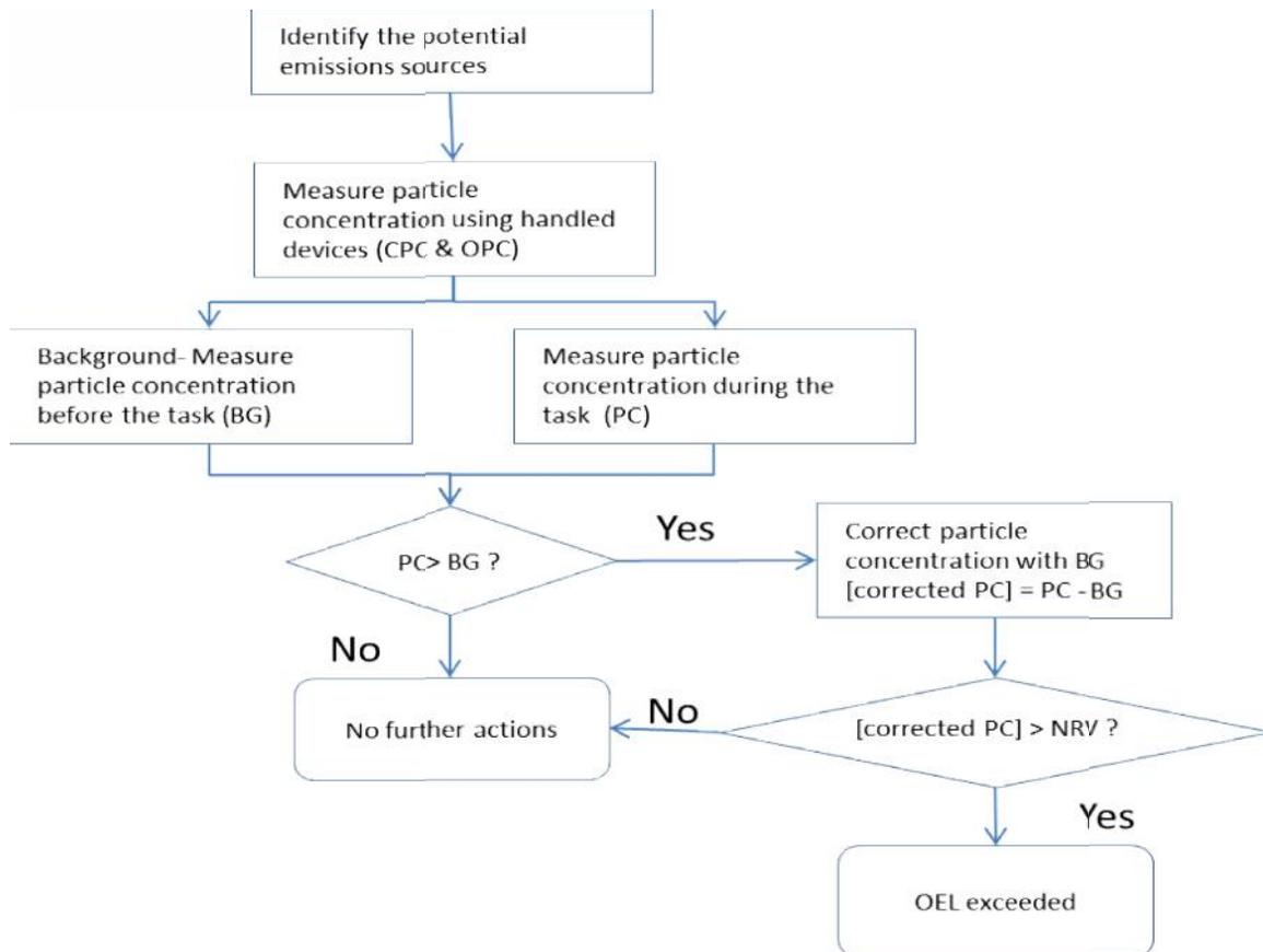
Figure 8. Flowchart describing the procedure to measure particle concentration (particles/cm<sup>3</sup>).
