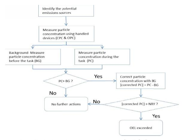
Figure 8. Flowchart describing the procedure to measure particle concentration (particles/cm3).
