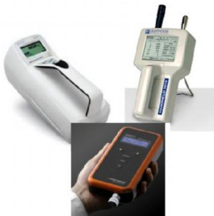
**Figure 7. Picture of portable CPC3007, OPC and DISCmini.**
